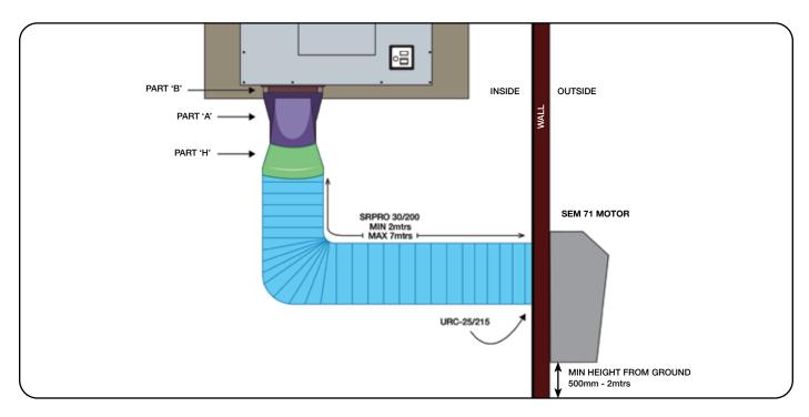
STEP 6B: Ducting to SEM 81 motor (200mm ducting)
