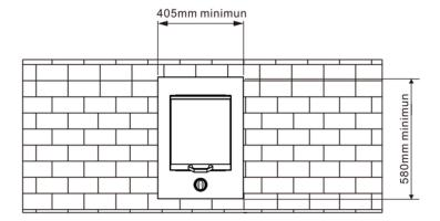
BBQ Sits Directly Onto Cabinetry Recommended Cut Out Dimensions: (w) >405mm x (h) 580mm x (d) 164mm
