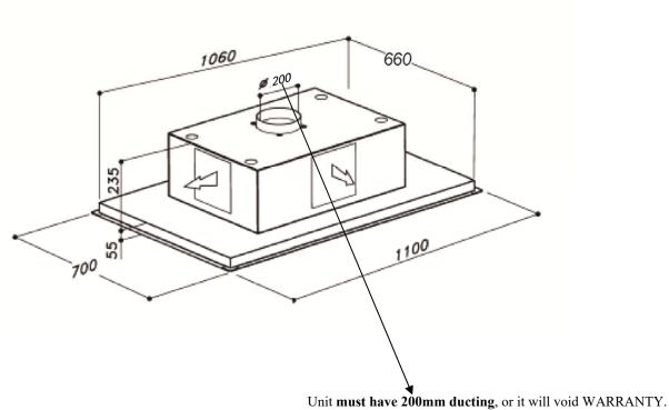
one must have 200min ducting, of it will void writed ivil.
